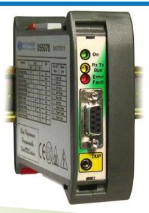
The DS5x two phase stepper motor drives series is composed of 27 different models, divided in 9 power sizes and 3 different interface types: DS50→RS485, DS52→RS232, DS54→USB. The communication interface is insulated from the power supply to grant reliability and noise immunity.
